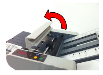
2.2 Push the fed roller shaft towards the right cover (near the control panel).
