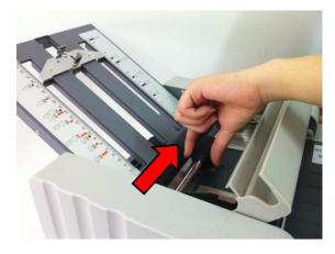
2.3 Push till one end is disengaged with the machine, lift the other side and remove the feed roller shaft.
