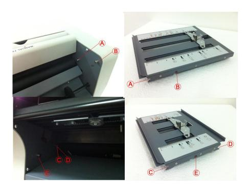
The lower plate is inserted in different directions for single fold and other folds.
