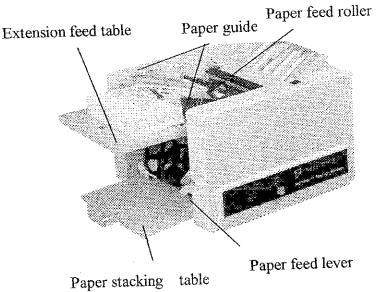
4.3.3 Adjust paper guide on left and right side so that it can touch the paper guide lightly. Set the center of paper to align the paper feed roller.
